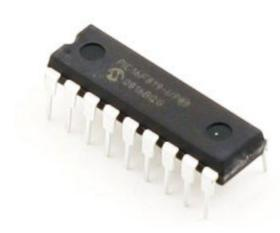
PIC controller with v,1.4 firmware
